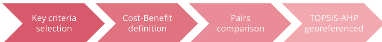
Figure 52 Methodological steps to identify candidate areas to install ECHO TES in specific case study.
