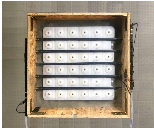
Figure 3-19: Radiant floor structure with PCM above (a) and under (b) piping; view of the lab-scale set-up (c).
