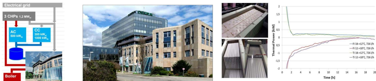
Figure 3-10: Installed TES capacity 10 \text{ m}^3 +15°C PCM solution providing total 440 kWh [5].
