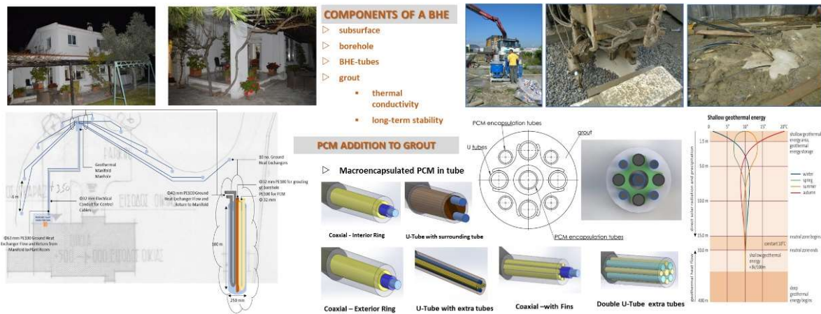
Figure 3-25: PCM addition for geothermal borehole grout for a small building in Cyprus.
